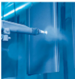
Coating treatment of external surface
